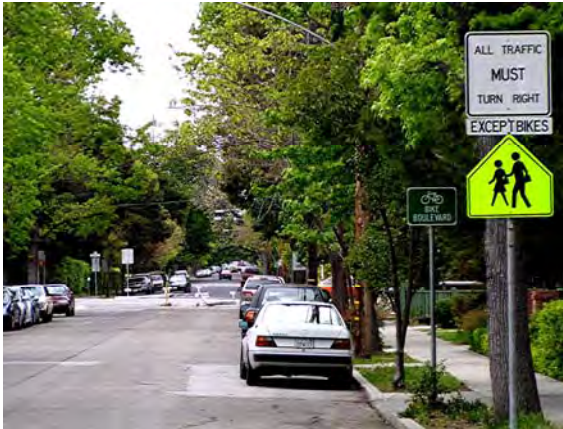
Figure 5.4 A non-motorized only crossing forces motor vehicles to turn at an intersection
