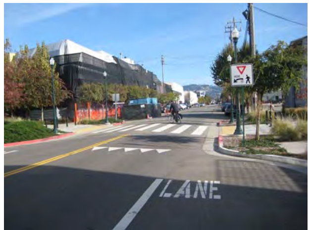
A Yield Controlled Crossing in Emeryville, California
