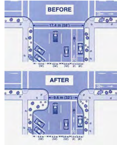
Curb Extensions - Before and After
